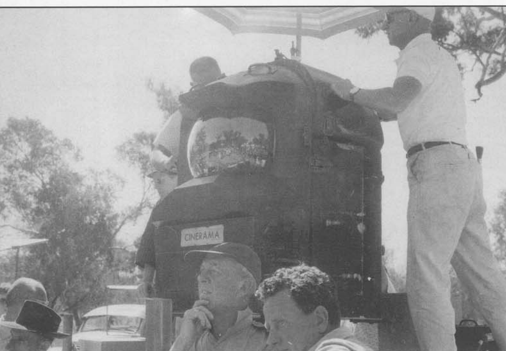
Filming Maori dancers, North Island, New Zealand in November 1957 with Cinerama camera number 6. The camera is fitted with a huge blimp to limit the camera noise. (Archive photo courtesy John McLean, Fifth Continent Music Pty, Australia).
