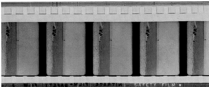
Figure 3. A print on nitrate stock showing conflicting identifications printed through from a safety master positive and a safety duplicating negative.
